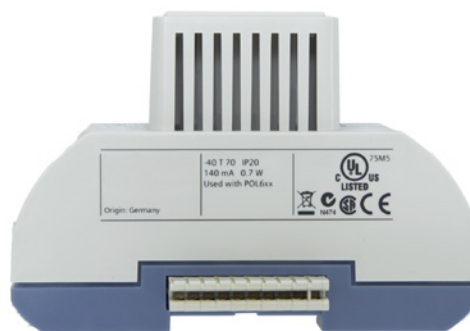
Figure 5: Communication Module with Board-to-Board Connector Inserted
